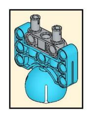
As you place this, tuck cables away in the space between the motors and the blue beam.
