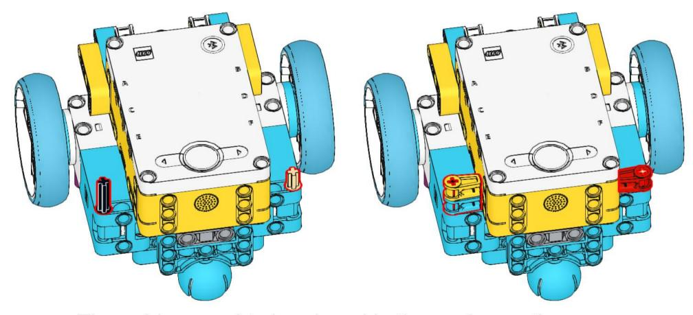
The cables need to be placed in these clasps, then onto the axle pins. Tuck all excess cable underneath robot
